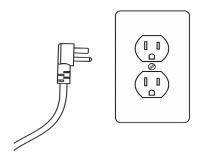
For hardwired installation - cut off the power plug , then use the wire connector to connect to external power supply.
