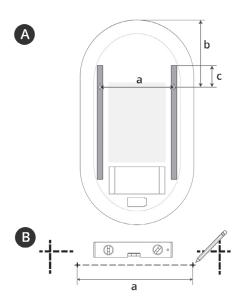
Predrill and install drywall anchors.
