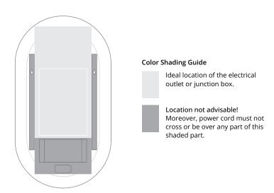
\*Diagram is for electrical outlet located behind the mirror. If electrical outlet is to the side or at the bottom/top of the mirror, always consider the length of the power cord (see previous page for measurement) and the darker shades in these diagrams where cord and/or plug must not cross over or be on top of.
