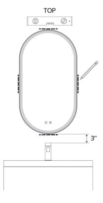
Measure the center of the holes (A) and mark the drilling locations. Ensure the mirror is level (B).
