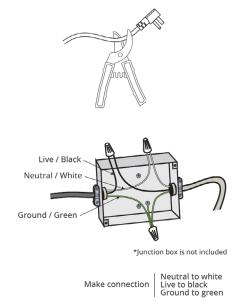
Both installation options can be connected and controlled with a light switch.
