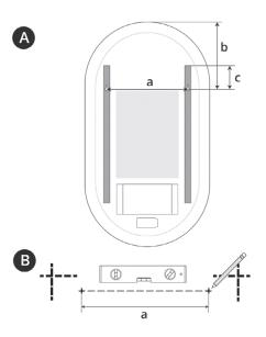
Predrill and install drywall anchors.
