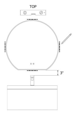
Measure the center of the holes (A) and mark the drilling locations. Ensure the mirror is level (B).
