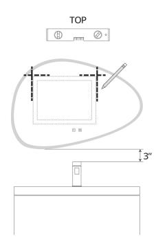
Because of the irregular shape, it is advisable to use the aluminum support at the back to mark/level the position of the mirror on the wall.
