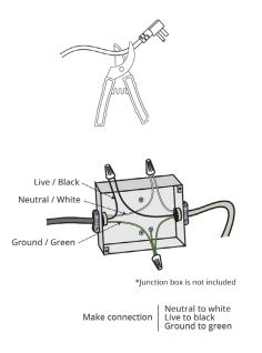
Both installation options can be connected and controlled with a light switch.
