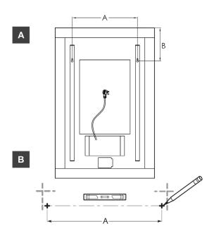
Predrill and install drywall anchors.
