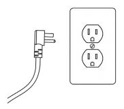
For hardwired installation - cut off the power plug, then use the wire connector to connect to external power supply.
