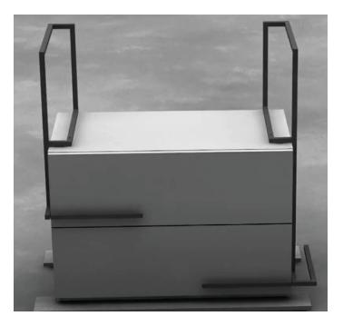
Add provided bolts to the threaded holes – only screw these in partway.
