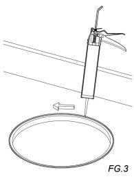
3. Apply a bead of silicone to the perimeter of the hole at the point at which the sink sits on the counter. *FG.3*
