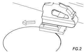
2. Cut out the counter -The cutting tools required will depend on the surface to be cut. FG.2 (Your sink comes with 4 mounting screws for mechanical fastening. Screws are only nesecary if for some reason silicone cannot be used. In this case, you will need to drill 4 holes in the counter to accommodate these screws)
